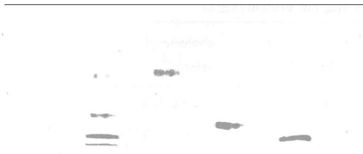
Fig 1 The LDL of the different oxidized degree were identified with the agarose gel electrophoresis. The concentration of the agarose was 0.5% and the electrophoretic solution was the barbital buffer solution, pH 8.6, 120v, 1h.
